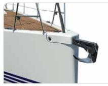
Standard GRP cowl with integrated anchor fitting
