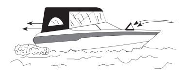
Figure 2.4 Desired Ventilation Through the Boat
