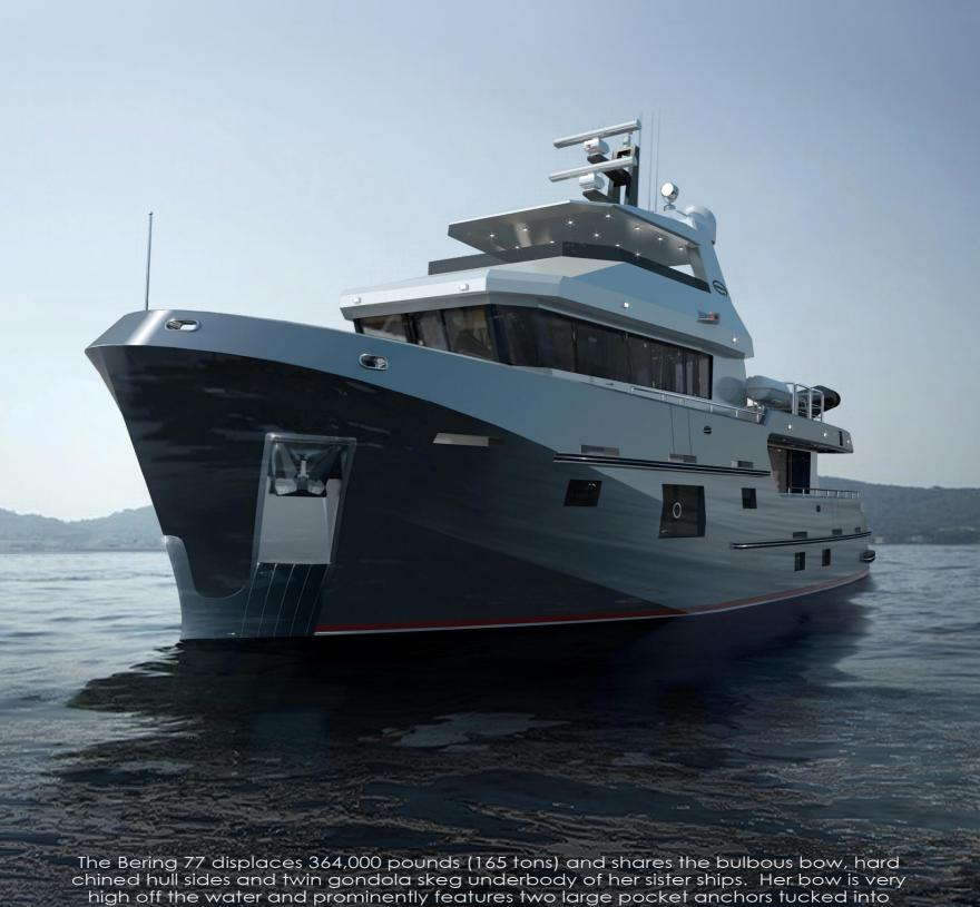
The Bering 77 displaces 364,000 pounds (165 tons) and shares the bulbous bow, hard chined hull sides and twin gondola skeg underbody of her sister ships. Her bow is very high off the water and prominently features two large pocket anchors tucked into the gorgeous stainless steel backing grill. This impressive bow height translates into a dry ride and creates very tall interior proportions allowing for over 7'2" (2 metres)
