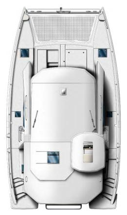
The Leopard 40 is available in either a 3 cabin, 2 head version, or a 4 cabin, 2 head version. Both layouts offer the option of additional storage, berth, or head in the forward hull.
