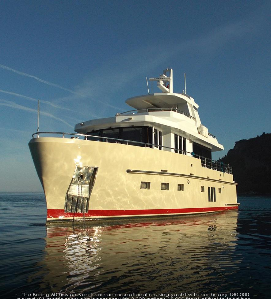
The Bering 60 has proven to be an exceptional cruising yacht with her heavy 180,000 pound (81 metric tons) displacement with 2,300 gallons (8,000 liters) of fuel to feed her efficient twin engine package provides her owners with excellent nonstop performance traveling thousands of miles with miserly fuel consumption to visit faraway destinations.
