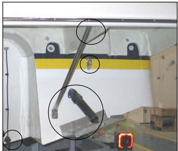
CHECK FOR TIGHTNESS & CORROSION
