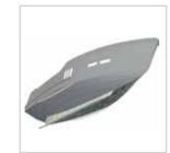
architect, Guy Saillard, has applied his vast experience in designing trawlers, to design the hull lines to carry a full load of 32 tonnes, while reducing drag and fuel consumption to a minimum.
